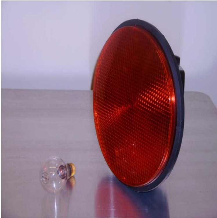
135 Watt bulb (left) used for 12" signal vs. 20 Watt LED 12" (right) signal
