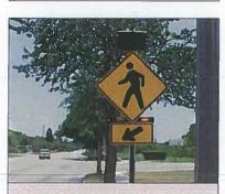
Figure 2: Activated, solar-powered, roadside RRFB at a mid-block crosswalk
